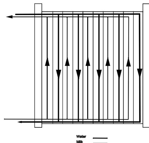
Figure 1: Single bank plate cooler
