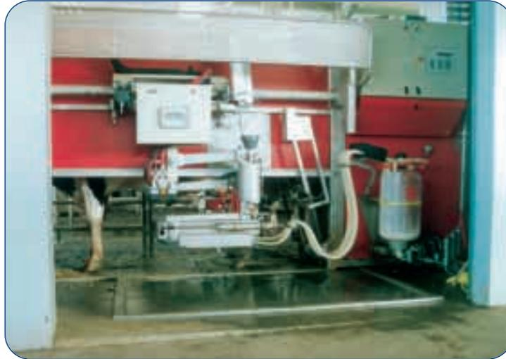
Figure 11.2: View of robotic milking system.
