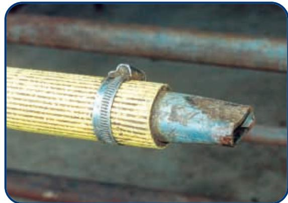
Figure 6.4: Flattened pipe making a simple nozzle on a yard cleaning hose.
