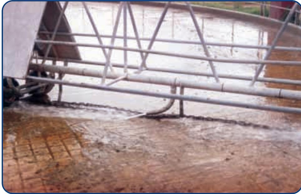
Figure 6.6: This system uses sections of chain and a number of water outlets on the backing gate.
